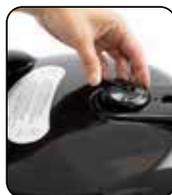
The Smart Canner comes with the Black Pressure Regulator (Jiggler) installed in cover on top of vent stem. Should you need to change to the Green Pressure Regulator (Jiggler) (for altitudes higher than 1,000 ft.) Simply lift the Pressure Regulator (Jiggler) straight up and pull off. To put the Pressure Regulator (Jiggler) back on the unit, simply put back on vent stem and push down.
